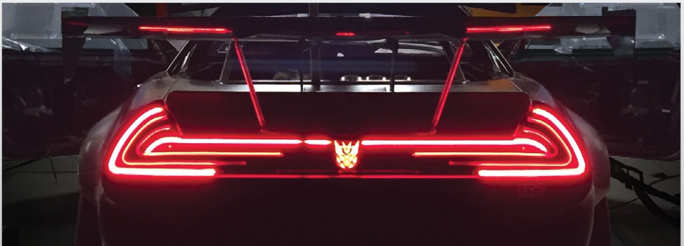
Fari posteriori, posizioni e stop, realizzati con kit "Red Tubes FPL/14R" Tail lights, position and brake, made with "Red Tubes FPL/14R"
